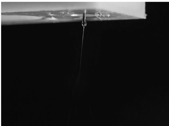
Fig.3. Image of polymeric nanofibers using electrospinning method. Results obtained for PVDF concentration  $c=20\%$ , applied voltage  $U=+12$  kV, distance between the capillary and collector  $l=120$  mm, and flow rate  $v=1$  ml/h in the air
