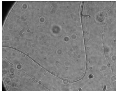
Fig.4. Optical image of a single PVDF fiber with a regular morphological form. The individual dots visible in the image are the impurities of the laboratory slide. Results obtained for capillary diameter  $d=0.5$  mm, applied voltage  $U=+12$  kV, distance between the capillary and collector  $l=120$  mm, and flow rate  $v=1$  ml/h in the air
