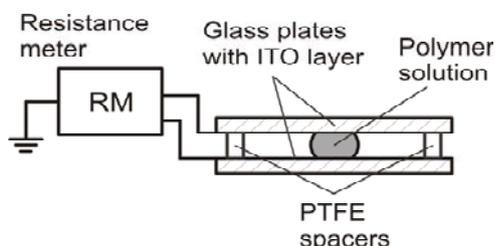
Fig.2. Scheme of the system for measuring the resistance of a polymer solution
