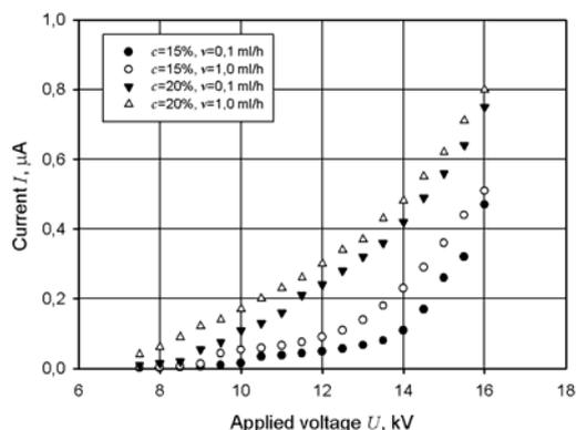
Fig.8. Current-voltage characteristics of electrospinning. Results obtained for capillary diameter  $d=0.5$  mm, distance between the capillary and collector  $l=120$  mm in the air
