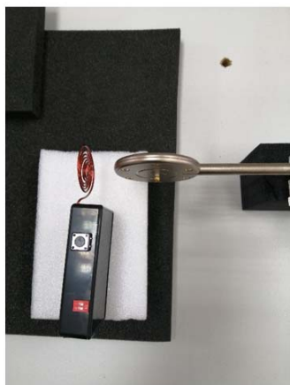
Fig. 8. View of a generator-tested located upstream of a D-dot probe
