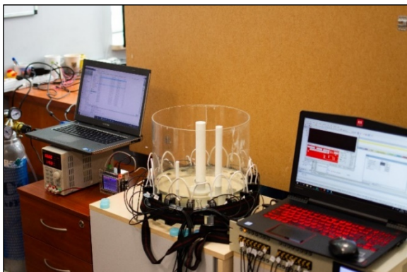
Fig.1. Test stand for UST+EIT hybrid tomograph [8]
