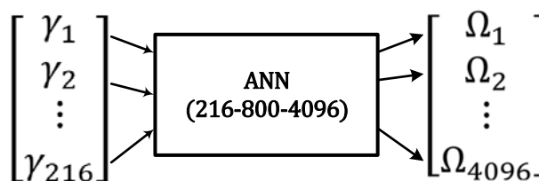
Fig. 4. The UST+EIT hybrid system converting 216 measurements with a single ANN
