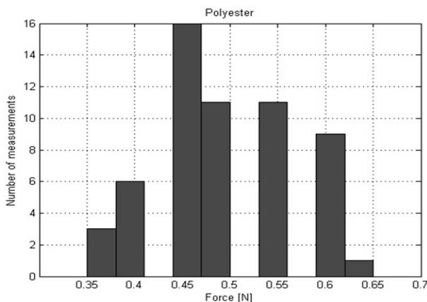
Fig. 5. Histogram showing the measurements of the polyester pull-off force.
