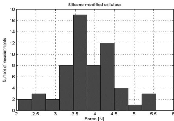
Fig. 4. Histogram showing measurements of the silicone-modified cellulose pull-off force
