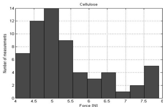
Fig. 3. Histogram showing the measurements of the cellulose pull-off force.
