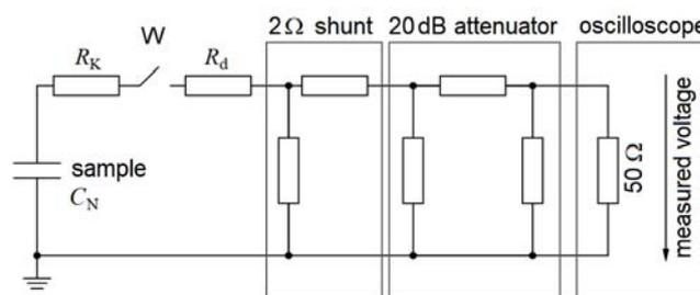
Fig. 1. The equivalent scheme of the measuring system for logging the discharge current-time characteristic during sample discharge, W – switch representing the occurrence of discharge (when closed)
