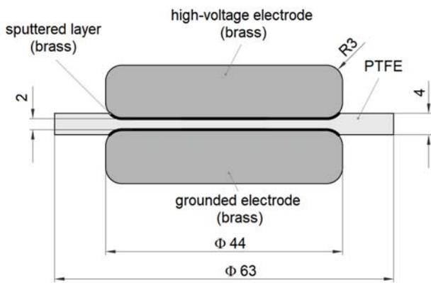
Fig. 2. Model of the reference capacitor
