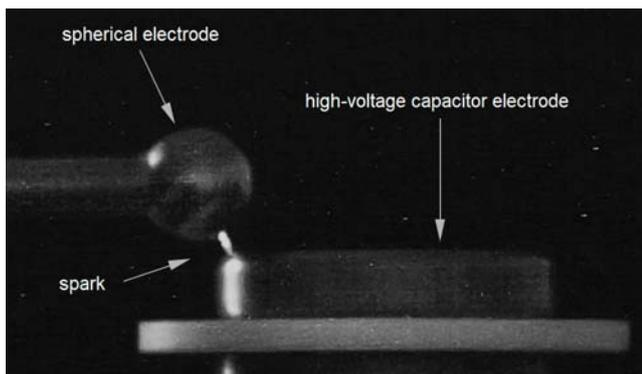
Fig. 3. Electrical discharge (i.e. spark discharge) from a surface of high-voltage reference capacitor electrode
