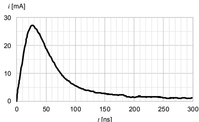
Fig. 6. Current-time characteristic during an ESD discharge from a charged dielectric fabric surface,  $R_d \cong 11$  k $\Omega$
