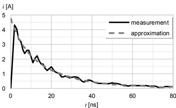
Fig. 4. Current-time characteristic of discharge from a surface of high-voltage reference capacitor electrode
