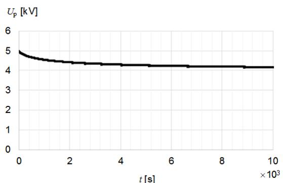
Fig. 5. Voltage-decay characteristic for reference capacitor
