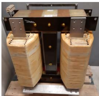
Fig. 5. The appearance of the special 3FR AN transformer before installation in the switchgear
