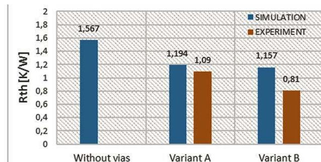
Fig. 9. Overview of thermal resistance (case - heatsink), multiple versions of IMS PCB
