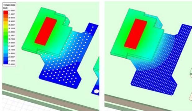
Fig.6. Thermal simulation of Insulated Metal Substrate PCB
