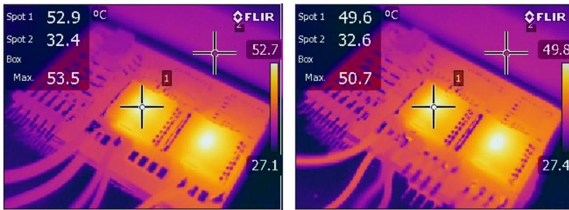
Fig.8. Thermal camera picture of IMS PCB - variant A (left), variant B (right). Spot no.2 represents the heatsink temperature.
