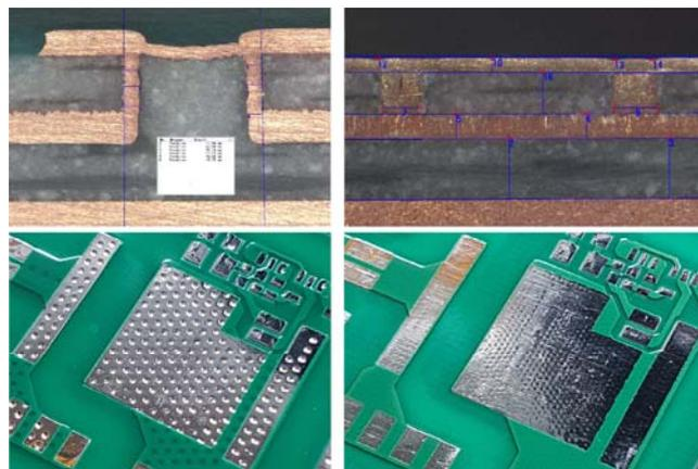
Fig. 7: Micro-section analysis and surface photos of tested prototypes - variant A (left), variant B (right)
