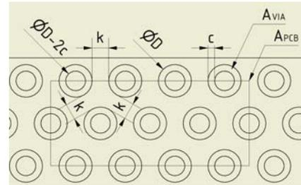
Fig.3. Parameters of printed circuit board thermal vias (top view)
