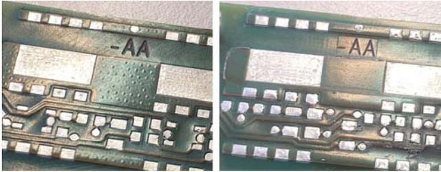
Fig.2. Surface view on six-layer PCB with filled and capped thermal vias (left) and copper inlay (right)
