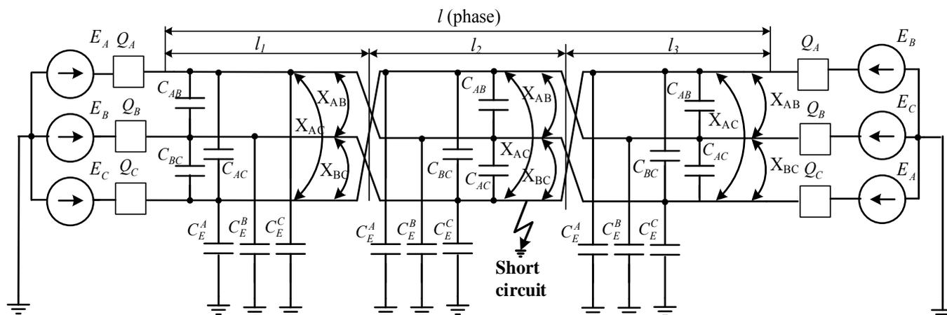
Fig. 6. Equivalent scheme for replacement of ultra-high voltage power line
