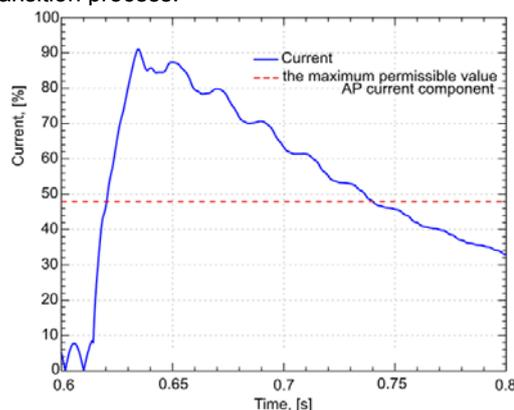
Fig. 2 Excess of ACC component the maximum permissible value
