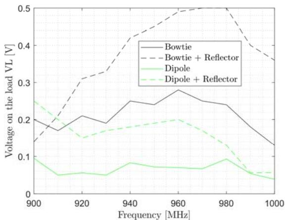
Fig.6. Voltage on the load, cross-polarization.
