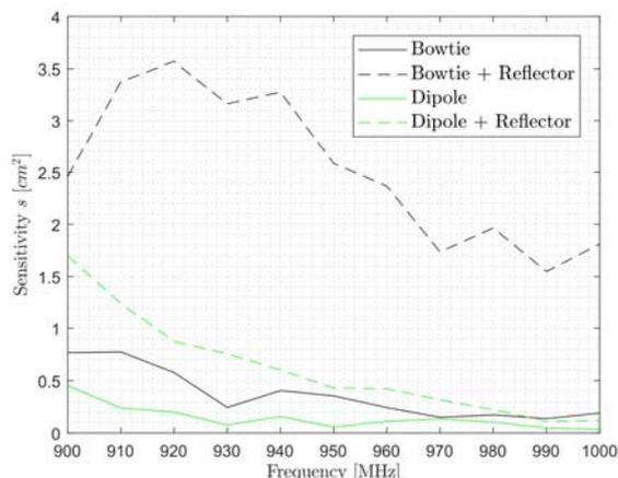
Fig.8. Sensibility  $s$  for the co-polarized case.
