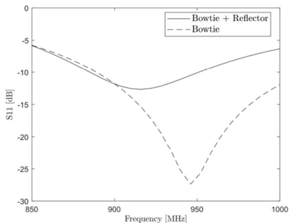
Fig.3. Computed return loss (S11) for the bowtie antenna, with and without reflector.
