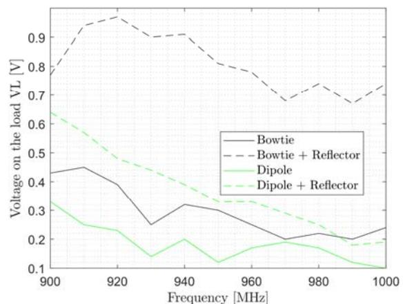
Fig.5. Voltage on the load, co-polarization.
