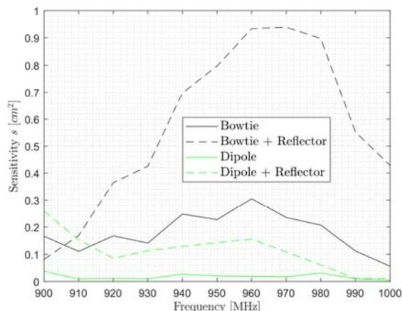
Fig.9. Sensibility  $s$  for the cross-polarized case.
