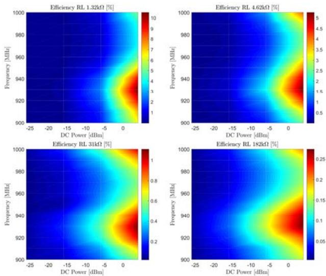
Fig.2. Circuit efficiency for  $R_L = 1.32 \text{ k}\Omega$  (top left),  $4.62 \text{ k}\Omega$  (top right),  $31 \text{ k}\Omega$  (bottom left) and  $182 \text{ k}\Omega$  (bottom right).
