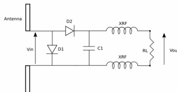
Fig.1. Circuit schematic of the voltage doubler and the antenna.
