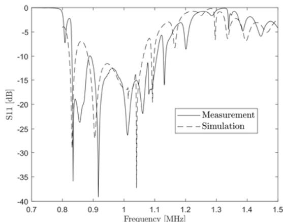
Fig.7. Open waveguide, measured and simulated return loss.
