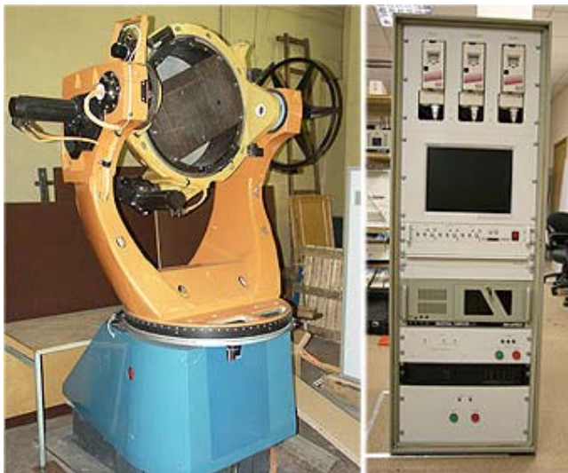
Fig. 2. Three-layer dynamic stand for semi-natural modelling (GosNIIAS)
