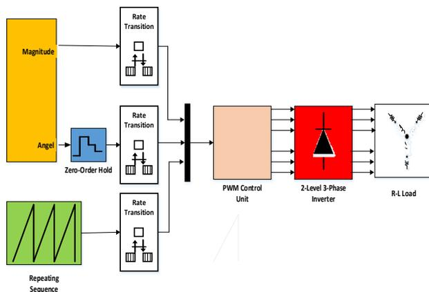
Fig.7. MATLAB/SIMULINK model of inverter and PWM controller
