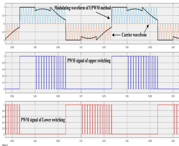
Fig.3. Carrier-based PWM of the UPWM method
