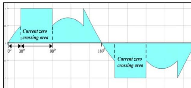
Fig.5. DPWM0 modulating waveform
