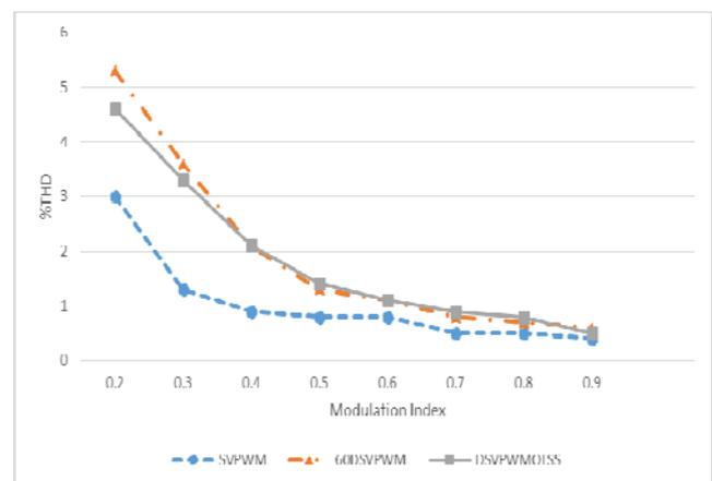
Fig.20. THD over the modulation index of SVPWM, 60DSVPWM and DSVPMOLSS methods at  $\cos \phi = 0.45$  (lagging)
