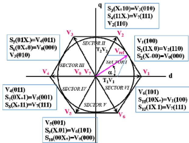
Fig.4. Voltage vectors of UPWM method
