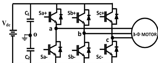
Fig.1. Two-level three-phase inverter
