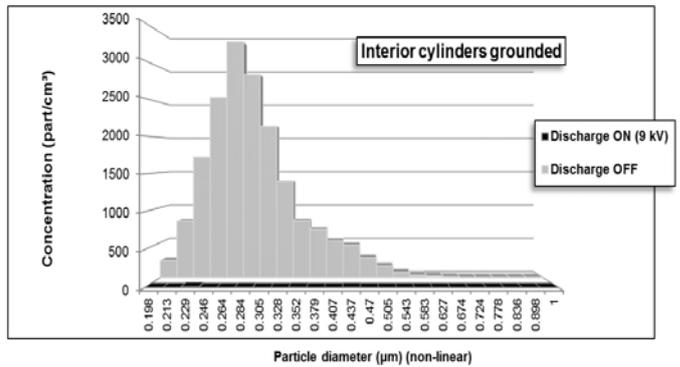
Fig.8.b. Granulometric Distribution of incense particles when the Interior cylinders are grounded
