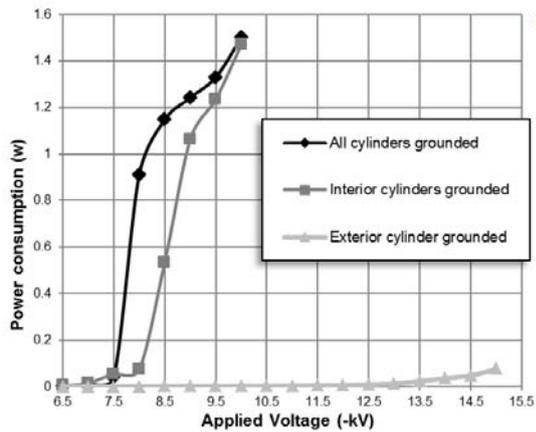
Fig.5. Power consumption versus voltage for negative corona discharges in the presence of particles.
