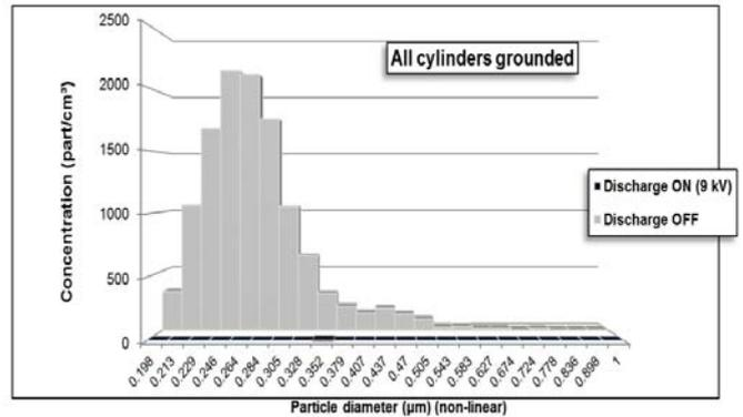
Fig.8.a. Granulometric Distribution of incense particles when All the cylinders are grounded
