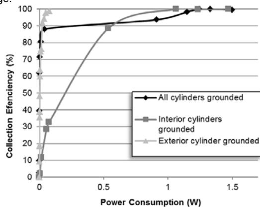
Fig.7. Particle collection efficiency as a function of power consumption for the three grounding cases.
