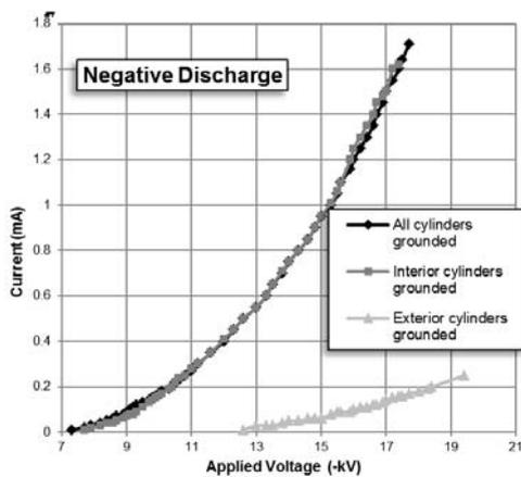
Fig.3.b. Current-voltage characteristics for negative corona discharges without particles.
