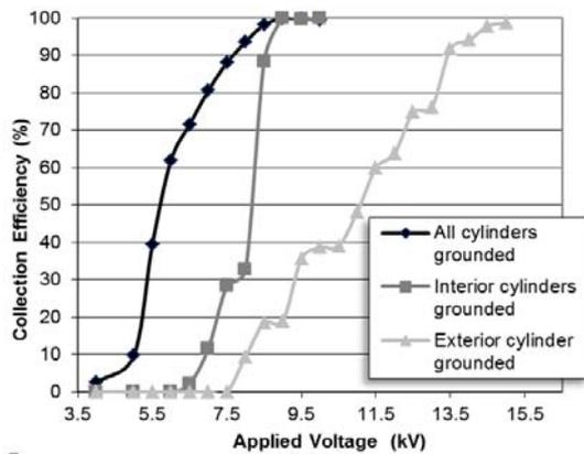
Fig.6. Particle collection efficiency as a function of the applied voltage.
