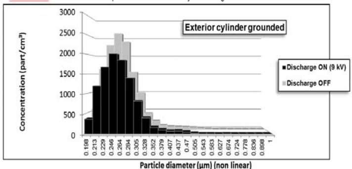
Fig.8.c. Granulometric Distribution of incense particles when the Exterior cylinder is grounded
