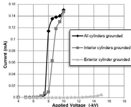
Fig.4. Current-voltage characteristics for negative corona discharges with the presence of particles.
