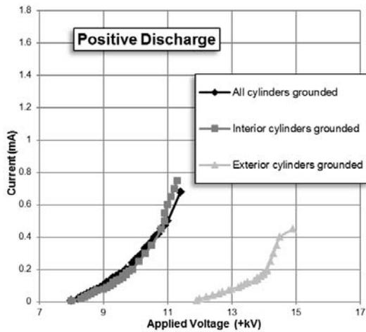
Fig.3.a. Current-voltage characteristics for positive corona discharges without particles.
