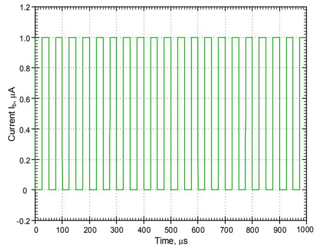
Fig.4. The bias current  $I_b$  for the sampling frequency  $f_s$  20 kHz
