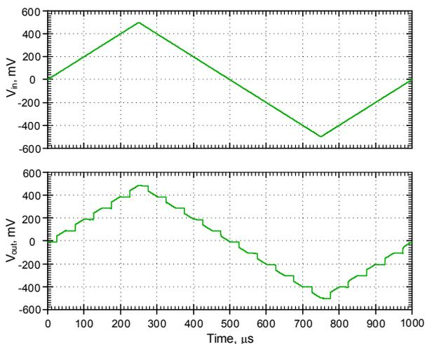
Fig.6. Simulated S/H output signal with triangular input by used sampling frequency in Fig. 4
