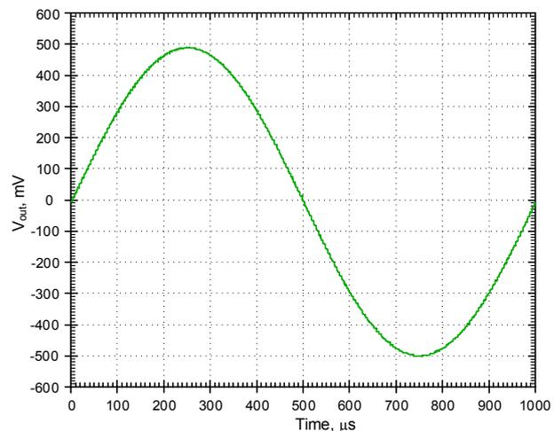
Fig.8. Simulated S/H output signal with sinusoidal input by used sampling frequency in Fig. 7
