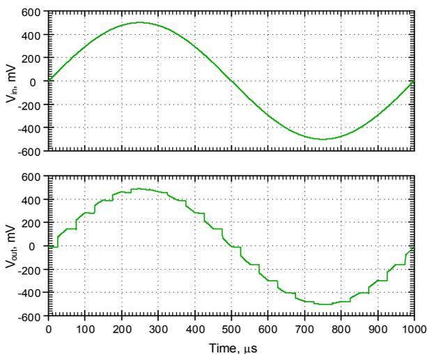
Fig.5. Simulated S/H output signal with sinusoidal input by used sampling frequency in Fig. 4
