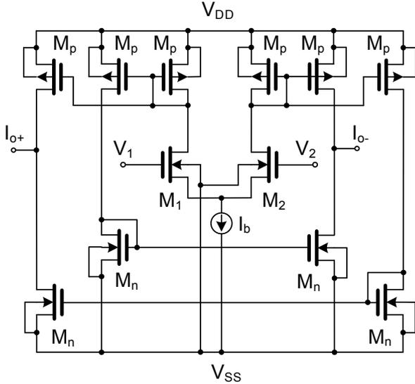
Fig.2. The schematic of dual-output OTA
