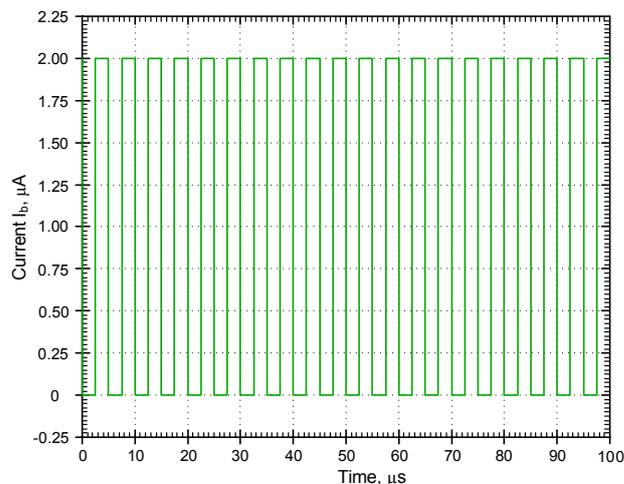
Fig.7. The bias current  $I_b$  for the sampling frequency  $f_s$  200 kHz
