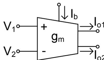
Fig.1. The circuit symbol of dual-output OTA
