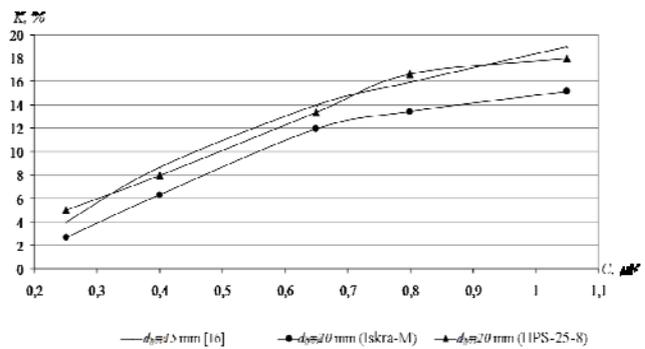
Fig. 2. Dependence of the grinding degree of Akbastau ore (up to 0.2 mm) on the capacity of capacitor batteries
