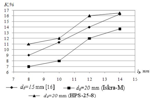
Fig. 3. Dependence of the grinding degree of Akbastau ore (up to 0.2 mm) on the discharge energy and on the interelectrode distance at the switching device of the TEPP
