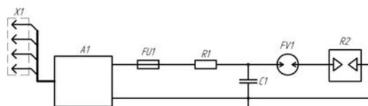
Fig.1. Block scheme of the electric pulse plant: A1 – a high-voltage power supply HPS-25-8, FU1 – a safety unit, C1 – a capacitor battery, FV1 – a commutation switch, R1 – a charging resistor (PEV-50-120), R2 – load or working channel, X1 – connector, a three-phase plug.
