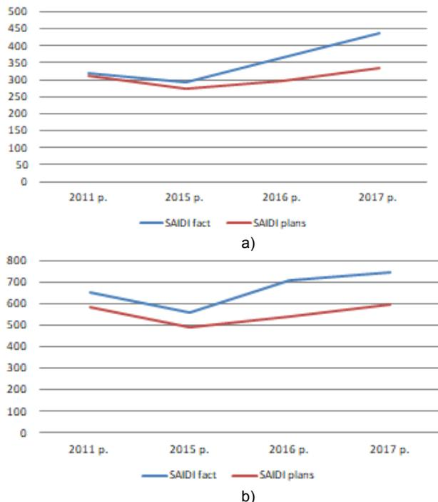
Fig. 2. Change of target indicator SAIDI (red curve) and actual (blue curve) for (a) urban electric networks; (b) rural electricity networks of the UES of Ukraine
