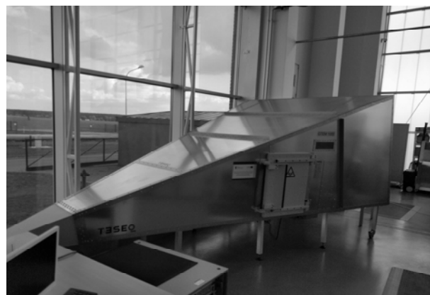
Fig. 1. A TESEQ GTEM 1000 cell for emission and immunity testing of electromagnetic disturbances
