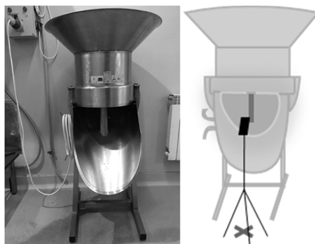
Photo 2. SZ-40 cabbage slicer with own design specifying the measuring point (own picture)
