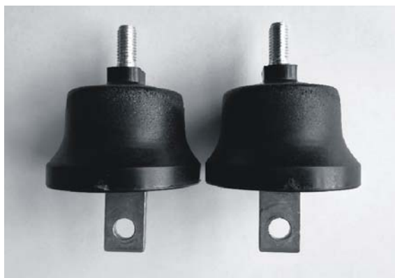
Fig. 2. Tested low voltage surge arresters with a polymer housing
