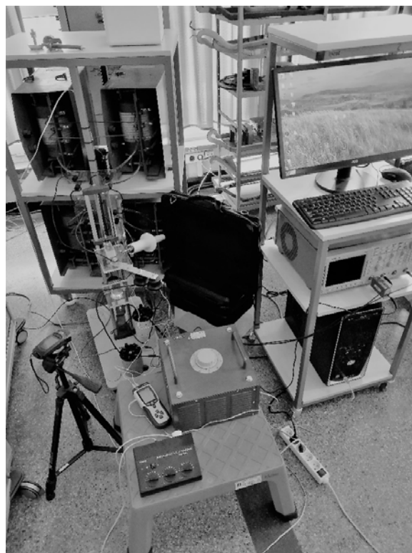
Fig. 4. Measuring stand for parallel-connected LV MOSAs tests - general view
