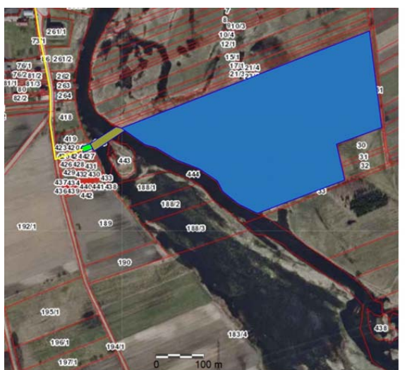
Key: reservoir area 105,000 m 2 (10.5 ha) volume of 630,000 m 3 parcel number 22.28 / 1 accumulation and hydropower facilities height of the bleed: 4.5 m, plot number 34.213, 22.444 transformer station parcel number 34.420-34.424 power output from the power plant line 15 kV to the nearest MV / LV station
