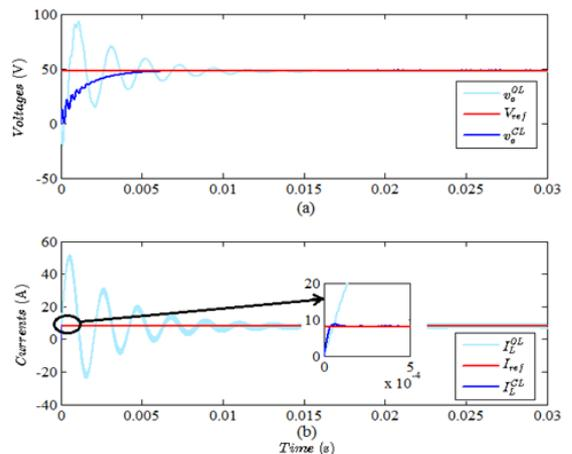
Fig. 4. Output voltage (a) and inductor current (b) waveforms for open loop and closed loop system
