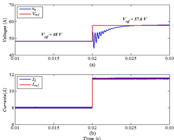
Fig. 5. Output voltage (a) and inductor current (b) waveforms for step change in  $V_{ref}$ .
