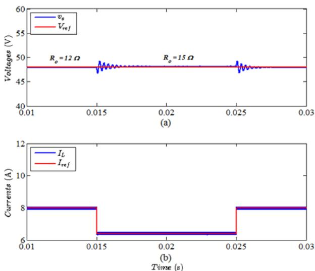
Fig. 7. Output voltage (a) and inductor current (b) waveforms for step change in  $R_o$
