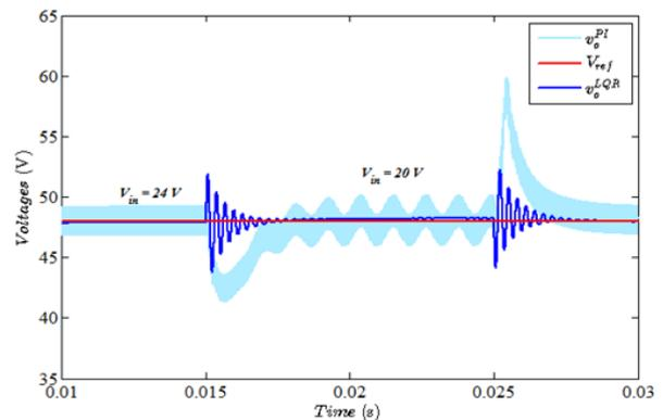
Fig. 8. Output voltage waveform for  $V_{in}$  variation
