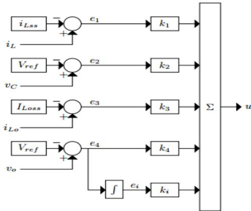
Fig. 3. LQR controller with integral action
