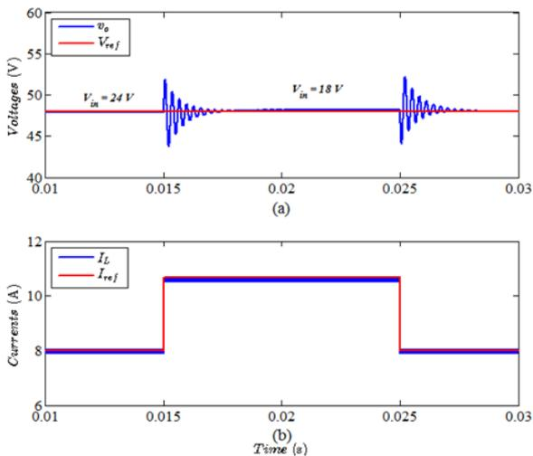
Fig. 6. Output voltage (a) and inductor current (b) waveforms for step change in  $V_{in}$ .
