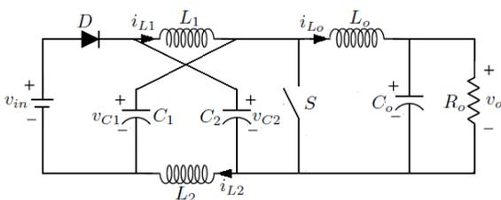
Fig. 1. Basic topology of Z-source DC-DC converter
