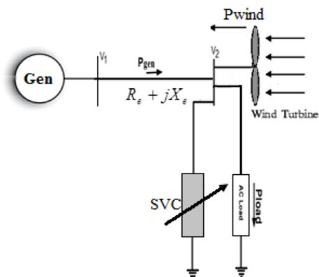
Fig. 1. SMIB equipped by SVC and wind turbine
