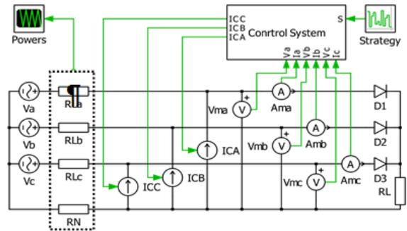
Fig. 3. Computer model of three-phase four-wire power system
