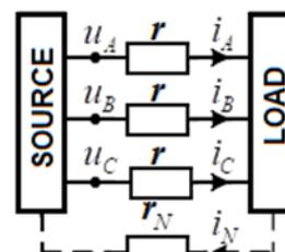
Fig. 1. Three-phase power supply system with resistive model of the transmission line
