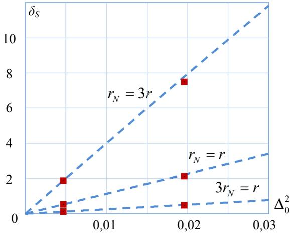
Fig. 2. Apparent power relative difference versus voltage zero-sequence factor under different values of transmission line resistances (dotted lines) and computer simulation results (□ marked pots).
