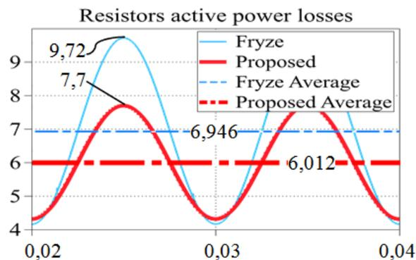
Fig. 4. Waveforms of instantaneous power losses and their average values
