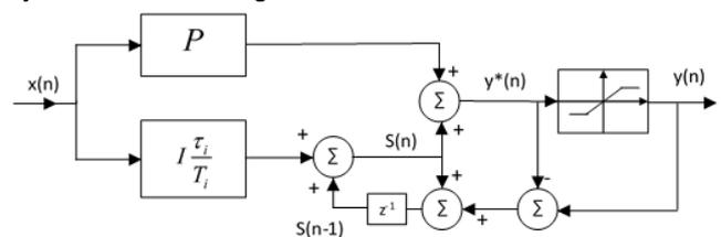
Fig.3. Discrete structure of the parallel PI controller
