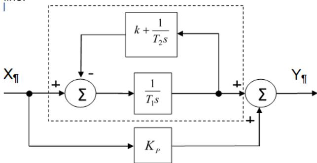
Fig.2. Proposed structure of the P+R controller
