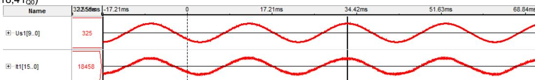
Fig.10. The waveform of voltage and current of the line in the unadjusted state of the controller frequency to the network frequency  $f_r > f_s$  (18458<sub>Q10</sub>=18,02<sub>Q0</sub>)
