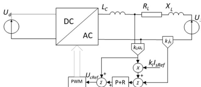
Fig.5. Diagram of the tested system
