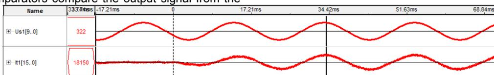
Fig.7. Device start-up, change of amplitude of preset current from 0 A to 13 A RMS (18150<sub>Q10</sub>=17,72<sub>Q0</sub>)
