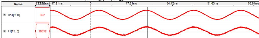
Fig.9. The waveform of voltage and current of the line in the unadjusted state of the controller frequency to the network frequency  $f_r < f_s$  (18852<sub>Q10</sub>=18,41<sub>Q0</sub>)
