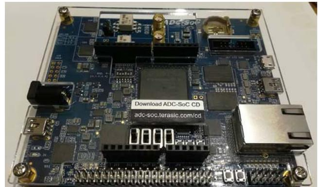
Fig.1. FPGA development board with Cyclone V 5CSEMA4U23C6N device.
