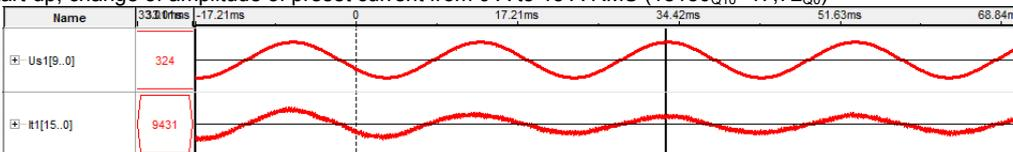
Fig.8. Change of set load from 13 A to 6.5 A RMS (9431<sub>Q10</sub>=9,21<sub>Q0</sub>)
