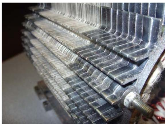
Fig.7. Stator before painting
