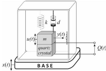
Fig. 1. Mechanical construction of the charge output accelerometer
