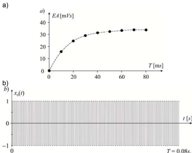
Fig. 2. a) Absolute error  $EA(x_0)$  vs. time  $T$ ; b) signal  $x_0(t)$  obtained for  $T=80$  ms
