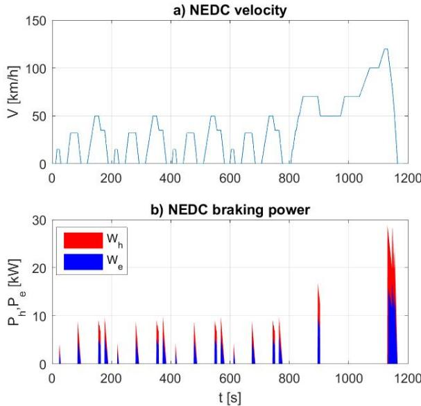
Fig. 8. a) Time history of vehicle speed in the NEDC test; b) Braking power division between frictional braking and regenerative braking (series braking)
