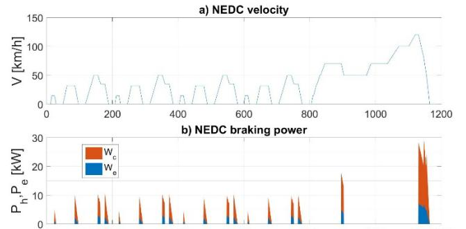
Fig. 13. a) Time history of vehicle speed in the NEDC test; b) Braking power division for the parallel braking in the NEDC test
