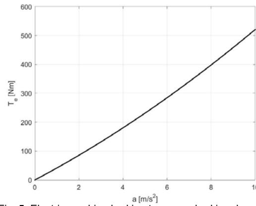
Fig. 5. Electric machine braking torque vs braking deceleration
