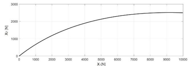
Fig. 3. Ideal braking force distribution curve ("I-curve") plotted for the data specified in Table 1.
