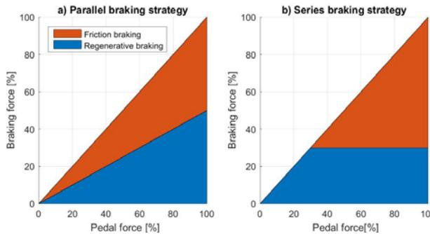
Fig. 4. Division of braking forces into frictional braking and regenerative braking: a) Parallel strategy; b) Serial strategy
