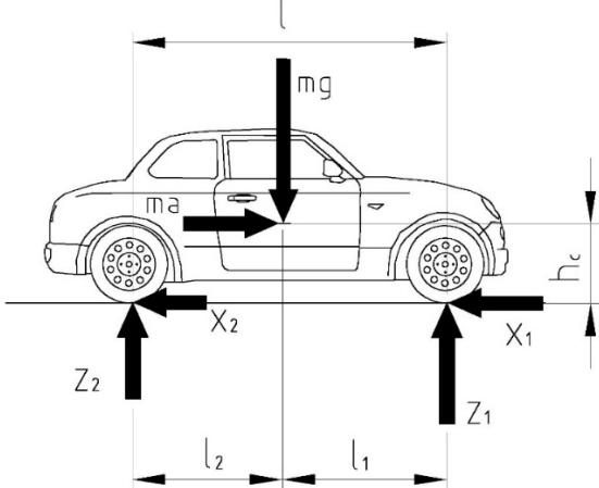
Fig. 2. Schematic presentation of the forces that act on a vehicle during the braking process.  $Z_1, Z_2$  – vertical reaction forces;  $X_1, X_2$  – horizontal forces;  $l_1$  and  $l_2$  – distances between the vehicle axles and the horizontal position of the centre of vehicle mass
