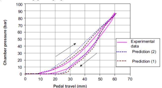
Fig. 10. Brake fluid pressure vs brake pedal travel curve [8]
