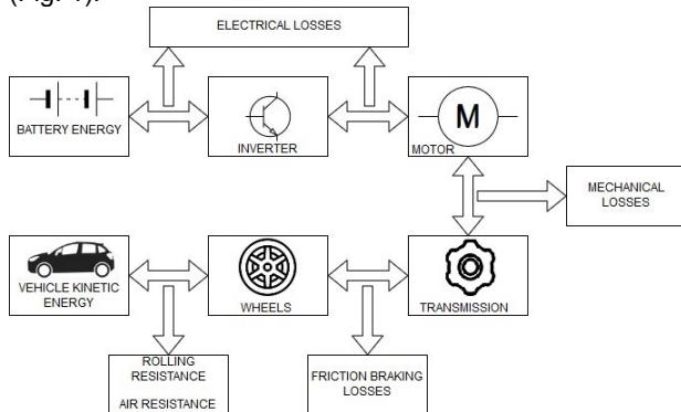
Fig. 1. Schematic diagram of the energy flows in an electric vehicle
