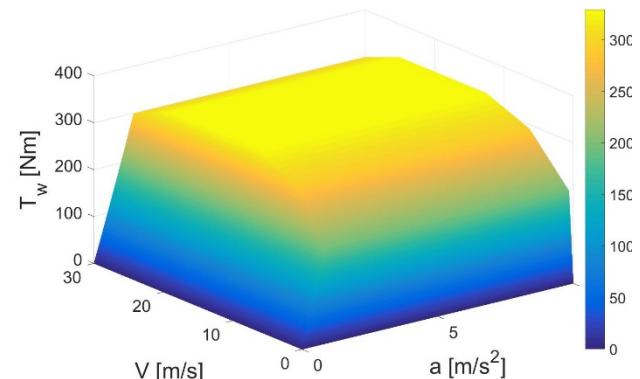
Fig. 7. Limitation of electrical braking torque on vehicle speed and braking deceleration:  $T_w$  – regenerative braking torque reduced to vehicle wheels
