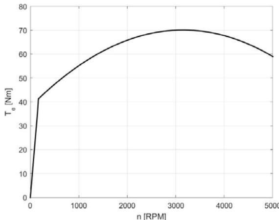
Fig. 6. Performance curve of the electric machine for the continuous generator operation mode:  $T_e$  – maximum braking torque of the machine;  $n$  – machine shaft speed
