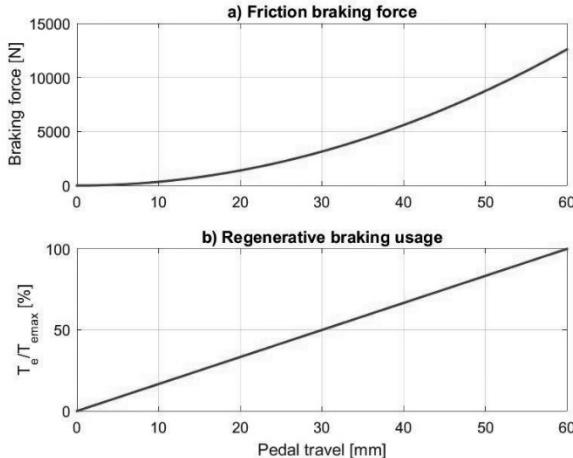
Fig. 11. a) Frictional braking force vs brake pedal position; b) Degree of utilization of the electric braking (ratio of the torque actually generated by the electric machine to the maximum braking torque obtainable from the machine at a specific operating point)
