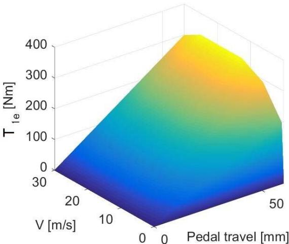
Fig. 12. Regenerative braking torque as a function of brake pedal position and vehicle speed
