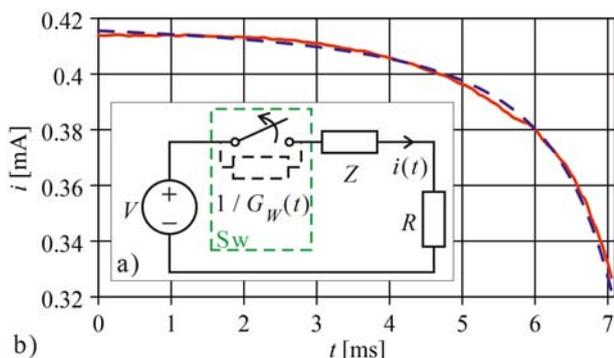
Fig. 4. Transient state in a circuit before the occurrence of conductance steps (ranges I and II in Fig. 1a): a) diagram of the circuit for the measurement of the current  $i(t)$ ; b) the measured current (red solid line) compared with the current calculated from equation (14) (blue dashed line)
