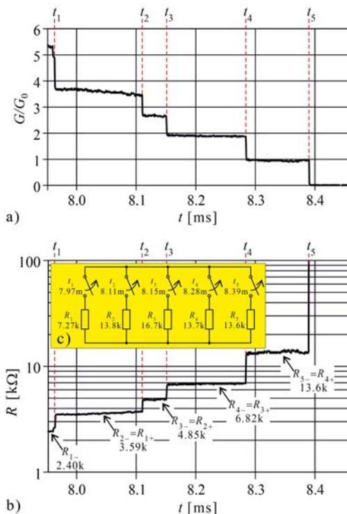
Fig. 3. Stepwise changes of the conductance and resistance of a stretched nanocontact: a) the last five conductance steps before the breaking of the nanocontact in range III in Fig. 1a; b) the corresponding time dependence of the nanocontact resistance; c) nanocontact model based on equation (12)
