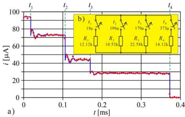
Fig. 7. a) Experimental current-time dependence (red diamonds) compared with theoretical characteristic (blue solid line) for the case when the circuit is periodic after the current steps. b) Model of mechanical switch used in the calculations
