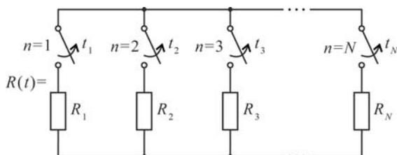
Fig. 2. Model of stretched nanocontact for range III in Fig. 1(a)
