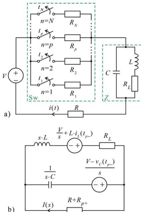
Fig. 5. Analysis of current in the circuit at the moment of opening of switch  $Sw$  in the phase where conductance decreases in steps as a result of nanocontact stretching between the terminals of the opening switch: a) diagram of the circuit used in the analysis; b) Laplace model of diagram a) after transformations
