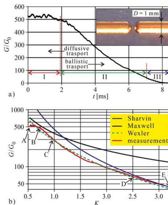
Fig.1. a) Conductance trace of the contact between the gold electrodes of an opening mechanical switch (see text for details). In the inset (top left), photograph of the electrodes of the mechanical switch used in the measurements. b) Calculated Sharvin, Maxwell and Wexler conductances vs. Knudsen number, compared with the dependence resulting from the measurement data presented in a) (see text for details)
