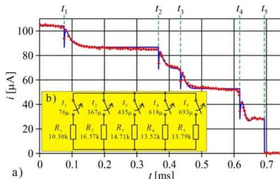
Fig. 6. a) Experimental current-time dependence (red diamonds) compared with the characteristic resulting from the theoretical analysis (blue solid line) for the case when the character of the circuit changes from aperiodic to periodic (at time  $t_{4+}$ ) as a result of a stepwise decrease in conductance. b) Model of mechanical switch used in the calculations
