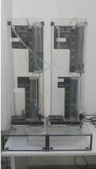
Fig. 1. Quanser's quadruple tanks system.
