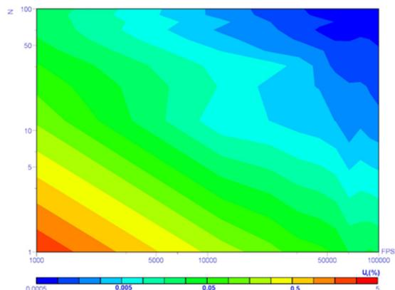
Figure 3 - uncertainty  $U_c(\omega_i)$  of the method shown as the percentage of the value (confidence level  $P=95\%$ , t-Student distribution value  $k=2.32$ ) when calibrating the speed sensor at 1000 rpm
