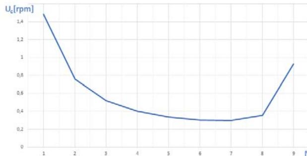
Figure 5 - total uncertainty  $U_c(\omega)$  versus N value after including the t-Student distribution for 1002 rpm speed measurement
