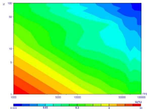
Figure 4 - uncertainty  $U_c(\omega_i)$  of the method shown as the percentage of the value (confidence level  $P=95\%$ , t-Student distribution value  $k=2.32$ ) when calibrating the speed sensor at 12000 rpm
