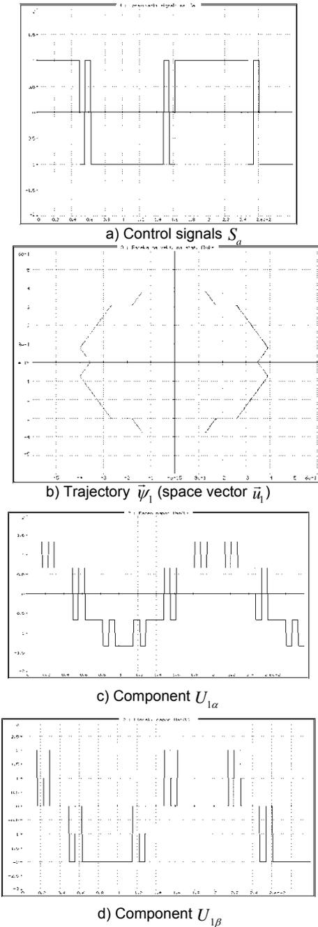
Fig. 3. Pulse edge space vector modulation  $V_p = \frac{f_{vkl}}{f_g} = 3$
