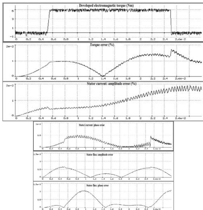
Fig. 5 Error assessment in direct vector control system (assumed:  $R_1$  change by 15%)
