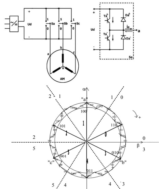
Fig. 1. VSI for DTC selecting the voltage vector for optimum stator flux trajectory
