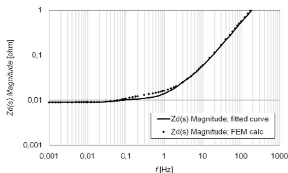
Fig. 2. Direct-axis magnitude impedance
