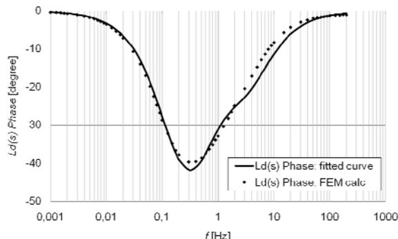
Fig. 5. Direct-axis phase inductance
