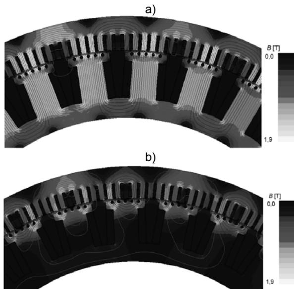
Fig. 13. Flux lines and distribution of magnetic induction at rated synchronous work for direct (a) and quadrature (b) axes
