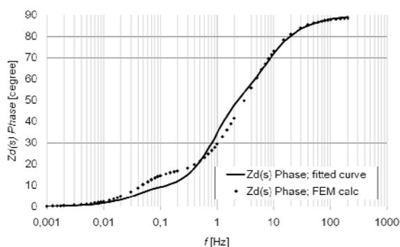
Fig. 3. Direct-axis phase impedance
