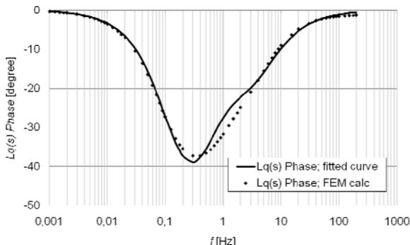
Fig. 9. Quadrature-axis phase inductance
