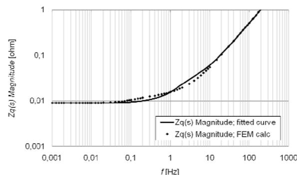
Fig. 6. Quadrature-axis magnitude impedance
