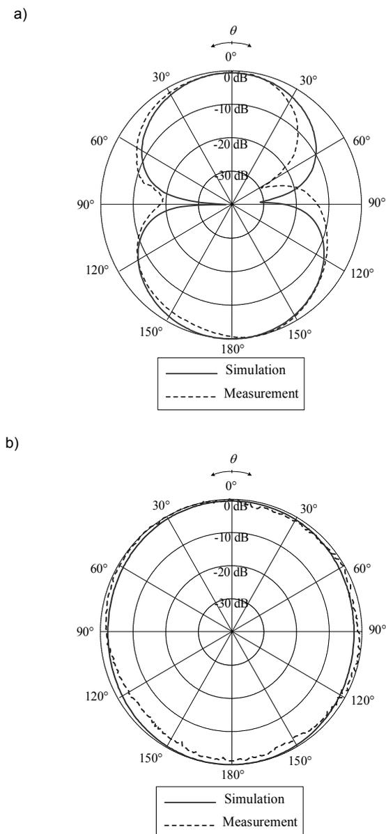
Fig.6. Radiation pattern at 2.45 GHz in: (a) xz-plane and (b) yz-plane
