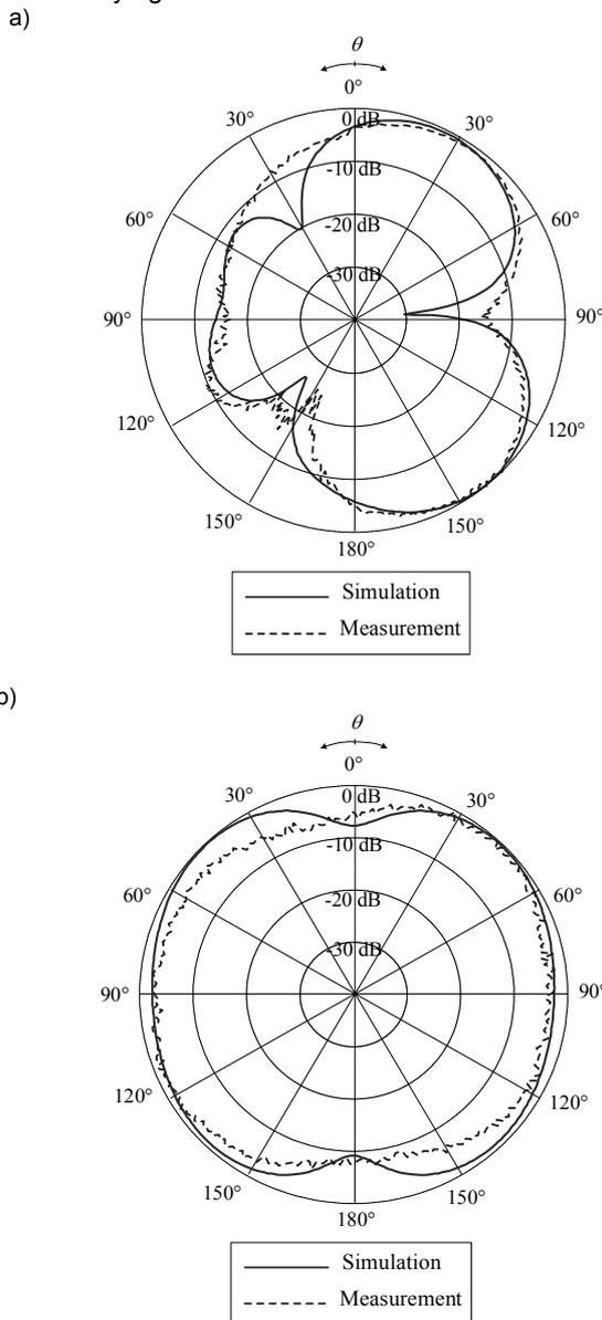
Fig.7. Radiation pattern at 5.5 GHz in: (a) xz-plane and (b) yz plane
