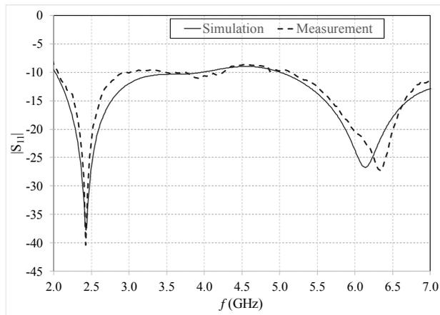
Fig.5. The simulated and measured  $|S_{11}|$  versus frequency
