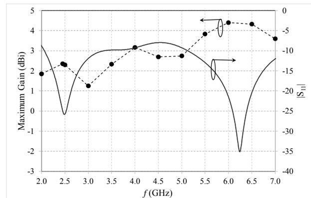
Fig.2. Maximum gain of proposed antenna for  $\alpha = 0^\circ$
