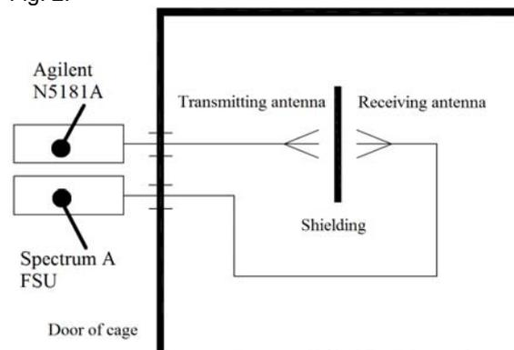
Fig.1. Workplace for purpose of measuring shielding effectiveness of electromagnetic field - block scheme
