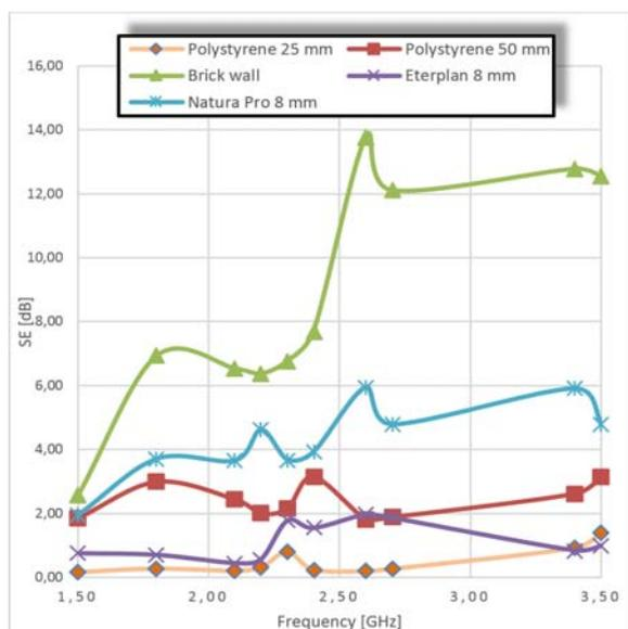
Fig.3. Shielding effectiveness for frequencies 1.5 GHz, 1.8 GHz, 2.1 GHz, 2.2 GHz and 2.3 GHz
