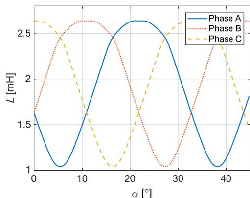
Fig. 3. Dependence of self-inductance of each phase vs. the rotor angle at a constant current value of  $I=35 A$
