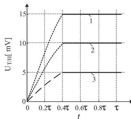
Fig.3. The time dependencies of the output voltage of the track and hold circuit for different ranges of RTD's resistance change: 1 – 15 Ω, 2 – 10 Ω, 3 – 5 Ω
