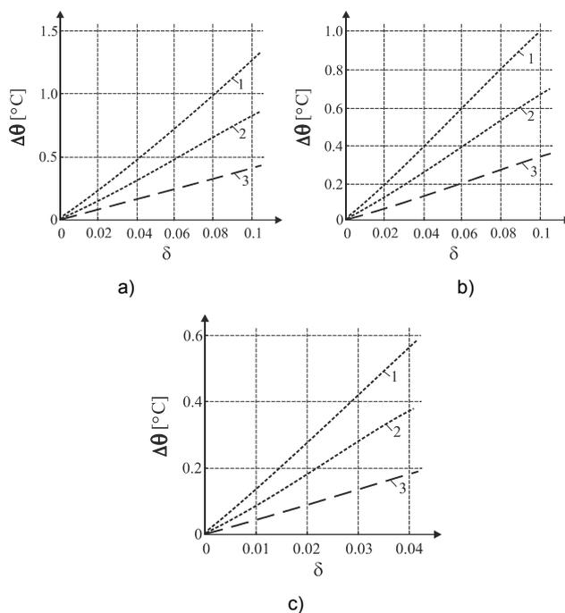
Fig.4. The dependencies of the absolute error of temperature measurement on the relative error of time interval formation for different values of resistance change in the measuring range: 1 – 15 Ω, 2 – 10 Ω, 3 – 5 Ω at  $t_m=0.4\tau$  (a),  $t_m=0.8\tau$  (b) and  $t_m=0.1\tau$  (c).
