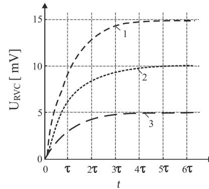
Fig.2. The time dependencies of the output voltage of the RTD resistance change-to-voltage converter for different ranges of RTD's resistance change: 1 – 15 Ω, 2 – 10 Ω, 3 – 5 Ω
