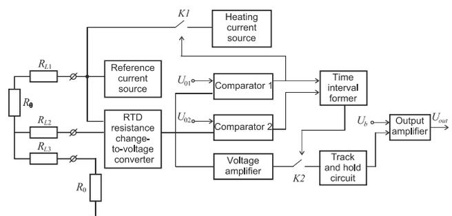
Fig. 1. Structural scheme of the thermoresistive transducer
