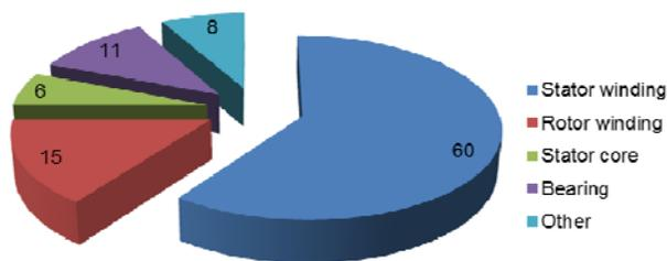
Fig. 2. The statistical data of SM failures
