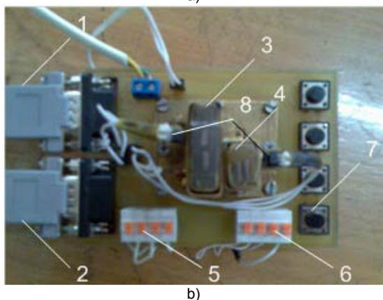
Fig. 4. The mobile variant of the system of automatic diagnostics of electrical steel:
