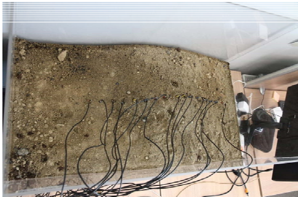
Fig.1. The physical model of the flood embankment with the arrangement of 16 electrodes
