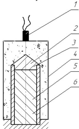
Fig. 3. The scheme of the explosive compaction of cylindrical samples: 1 – the detonator; 2 – the charge of the explosive; 3 – the generator of a plane shock wave; 4 – the shell for the explosive; 5 – a sample; 6 – a copper shell
