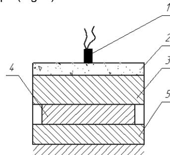
Fig. 5. The scheme of the explosive compaction by a repeated compression: 1 – the detonator; 2 – the explosive; 3 – the plate with a greater acoustic rigidity; 4 – sample; 5 – the plate with a lower acoustic rigidity
