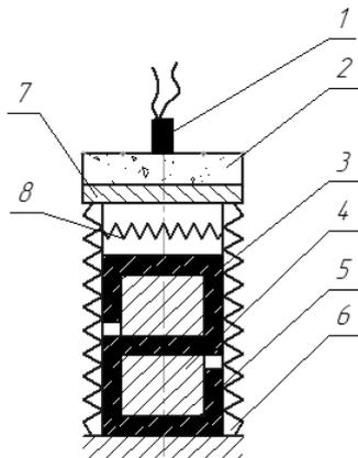
Fig. 4. The scheme of the compaction by throwing the striker: 1 – the detonator; 2 – the explosive; 3 – copper shell; 4 – samples; 5 – a copper shell; 6 – the corrugated support; 7 – the striker; 8 – the elastic screed
