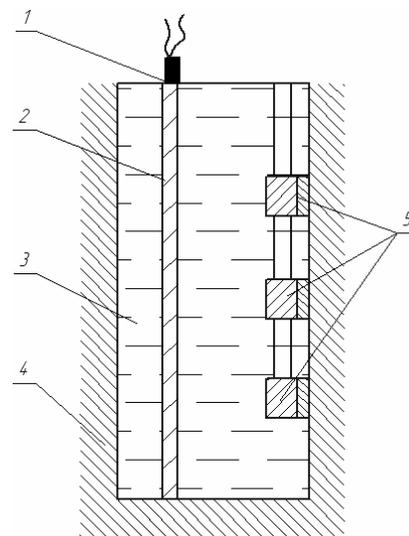
Fig. 6. The scheme of hardening in a closed volume: 1 – the detonator; 2 – the detonating cord; 3 – the transmission medium; 4 – the rigid walls; 5 – the compacted samples
