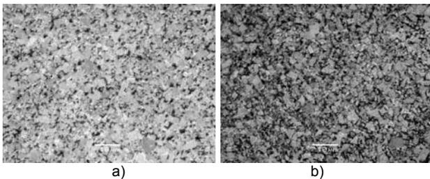
Fig. 7. Microstructures of the samples: a – sample made according to the serial technology; b – sample after a low-intensity impulse loading
