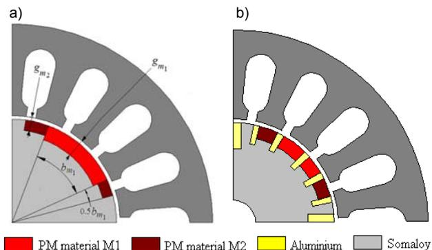
Fig. 2. New structures of PM synchronous motors with hybrid rotors
