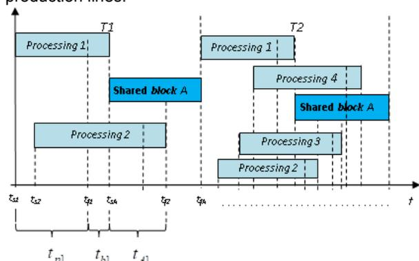
Fig.2. Chart for serial-parallel processing
