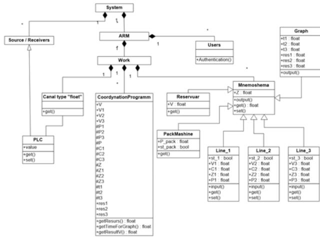
Fig.3. The UML diagram of the classes of the information technology of the control of the preparation and packaging of dairy products
