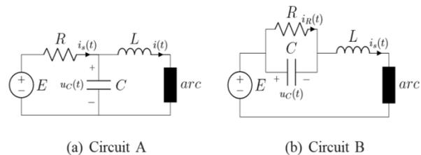
Fig. 1. Two typical electric arc circuits.
