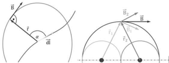
Fig.16. The graphical method of determining the magnetic field and their applications to arbelos.
