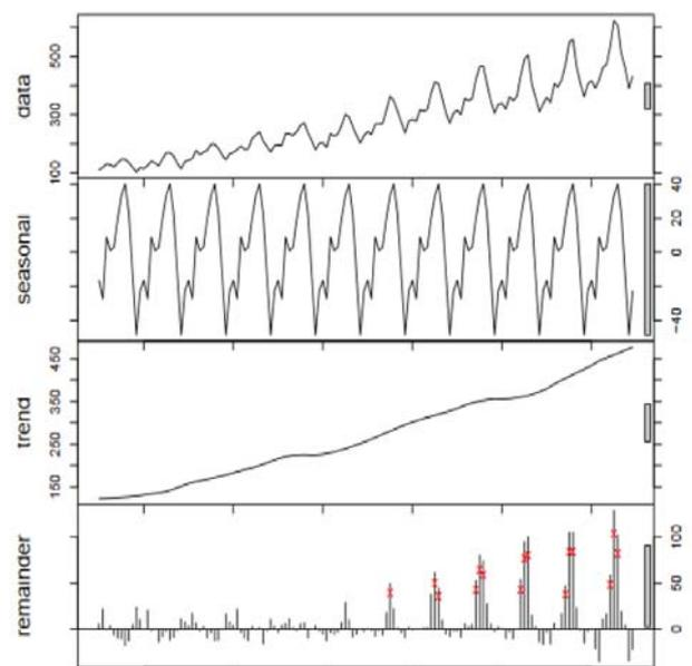
Fig.1 Decomposition of the data stream (successively from the top): the original data, seasonal fluctuations, trend and random fluctuations.
