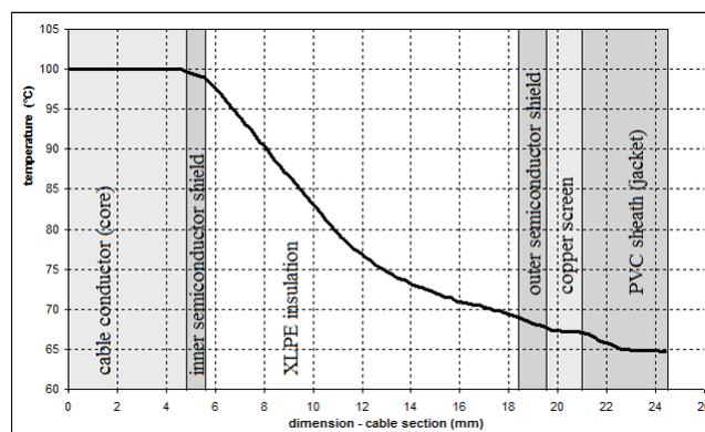
Fig.1. Temperature distribution in individual layers in XLPE 150 mm<sup>2</sup> 18/30 kV MV cable - simulated data in ANSYS
