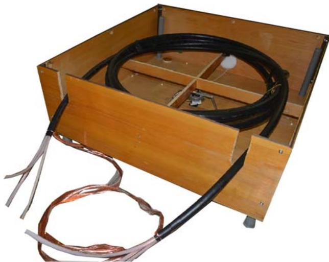
Fig.2. Open chamber for passive cable heating
