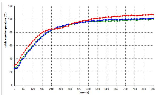
Fig.5. Warming characteristics of 150 mm<sup>2</sup> MV cable by 1 kA current
