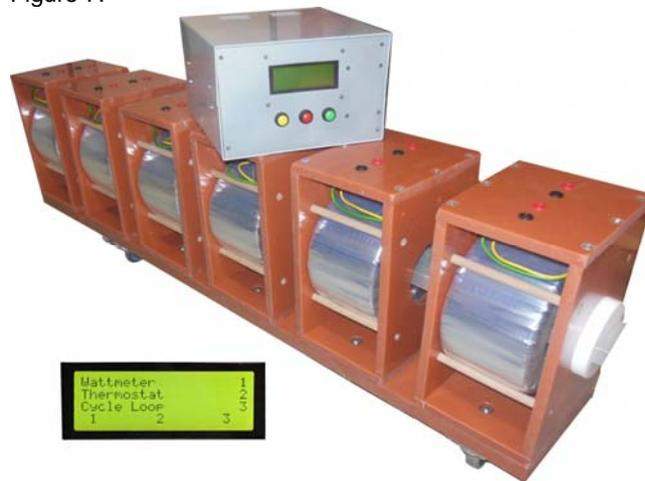
Fig.7. Autonomous system for heating MV and HV cables
