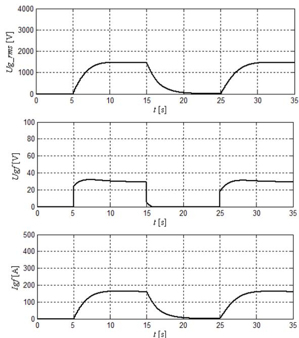
Fig.3. Simulation results for generator voltage stator windings in open-circuit mode of operation and given voltage changes in range 0-0.4 $U_N$ :  $U_{g\_rms}$  - generator RMS line-to-neutral voltage,  $U_{gf}$  - generator excitation voltage,  $I_{gf}$  - generator field current,  $I_{rms}$  - motor RMS stator current
