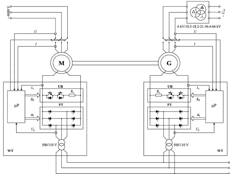
Fig.1. Block diagram of the machines set: M – synchronous motor, G – synchronous generator, WT - microprocessor-controlled power supply excitation unit,  $\mu P$  - microprocessor system, PT - thyristor rectifier, UR - start-up system,  $R_r$  – start-up resistor
