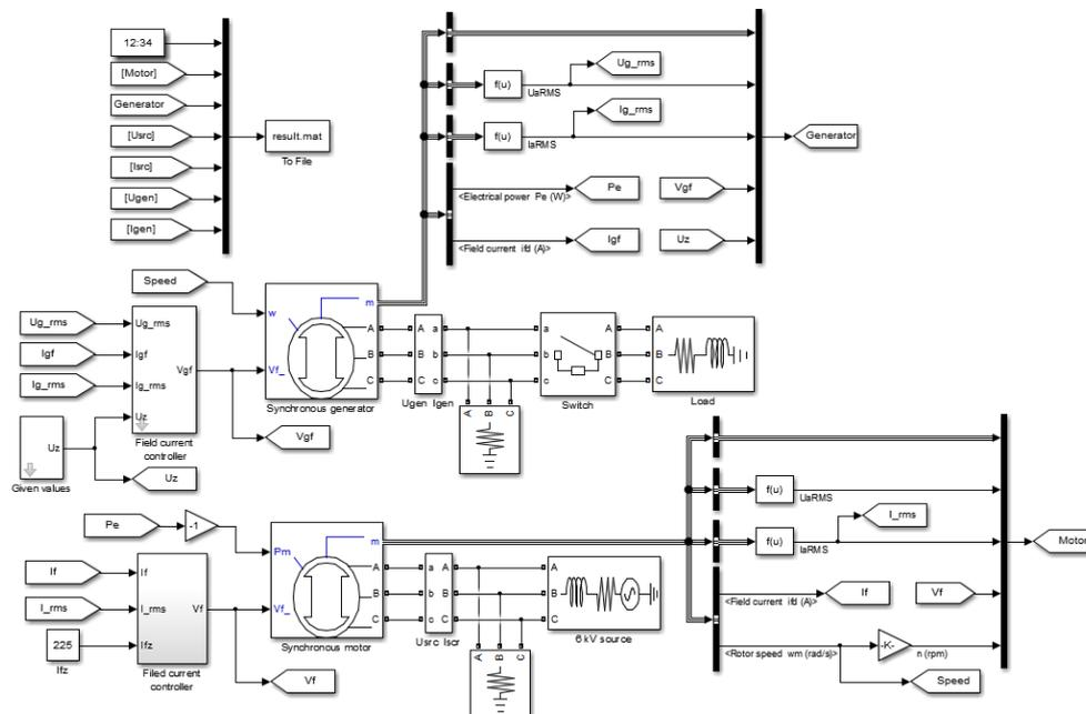
Fig.2. The simulation model of synchronous motor - synchronous generator machines set of Matlab-Simulink
