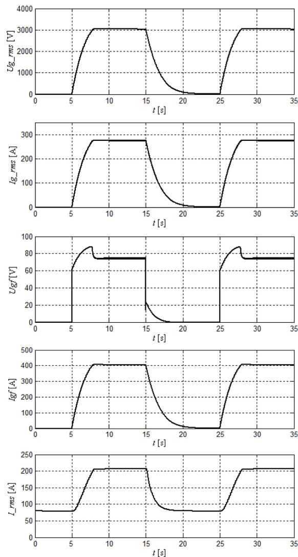
Fig.6. Simulation results for generator loaded by the RL type load and given voltage surges in range  $0-U_N$ :  $U_{g\_rms}$  - generator RMS line-to-neutral voltage,  $I_{g\_rms}$  - generator RMS stator current,  $U_{gf}$  - generator excitation voltage,  $I_{gf}$  - generator field current,  $L_{rms}$  - motor RMS stator current
