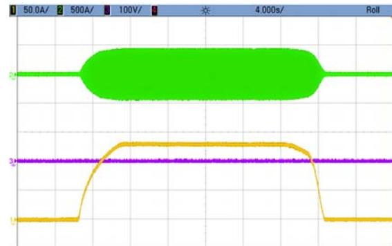
Fig.9. Measurements of the generator in the short-circuit stator windings mode of operation: 1 – field current, 2 – stator current, 3 - stator phase-to-phase voltage
