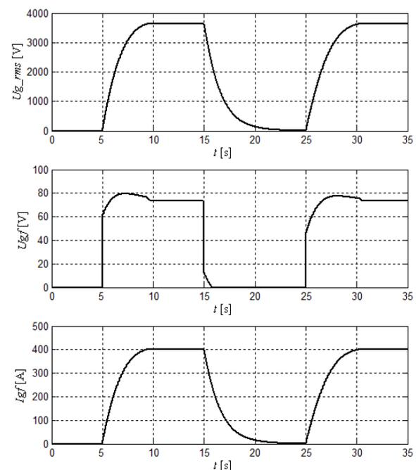
Fig.4. Simulation results for generator voltage stator windings in open-circuit mode of operation and given voltage changes in range 0- $U_N$ :  $U_{g\_rms}$  - generator RMS line-to-neutral voltage,  $U_{gf}$  - generator excitation voltage,  $I_{gf}$  - generator field current,  $I_{rms}$  - motor RMS stator current
