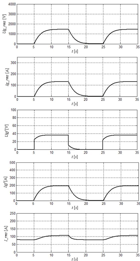
Fig.5. Simulation results for generator loaded by the RL type load and given voltage surges in range  $0-0.4U_N$ :  $U_{g\_rms}$  - generator RMS line-to-neutral voltage,  $I_{g\_rms}$  - generator RMS stator current,  $U_{gf}$  - generator excitation voltage,  $I_{gf}$  - generator field current,  $L_{rms}$  - motor RMS stator current
