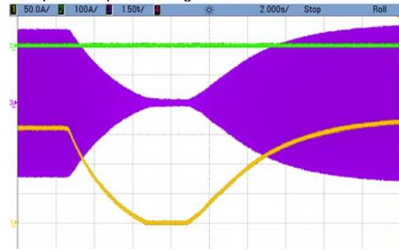
Fig.10. Measurements of the generator in the open-circuit stator windings mode of operation: 1 – field current, 2 – stator current, 3 - stator phase-to-phase voltage
