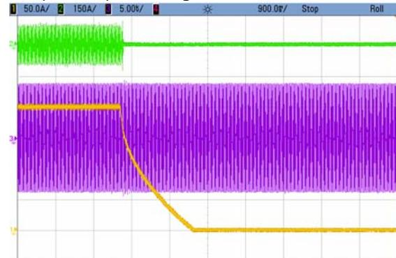
Fig.11. Discharging excitation circuit energy during engine shutdown: 1 – field current, 2 - stator current, 3 - phase-to-phase voltage at the switchgear station
