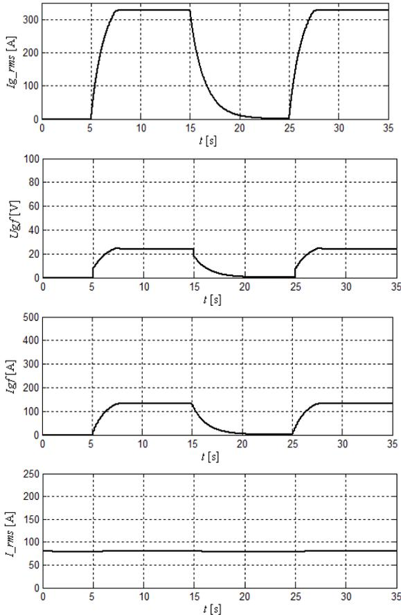
Fig.7. Simulation results for the generator stator windings in a short circuit mode of operation and given field current surges in range  $0.5I_{fn}$ :  $I_{g\_rms}$  - generator RMS stator current,  $U_{gf}$  - generator excitation voltage,  $I_{gf}$  - generator field current,  $I_{rms}$  - motor RMS stator current
