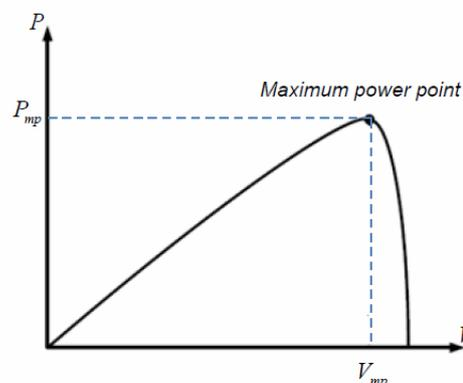
Figure 3: P-V curve for a PV module.
