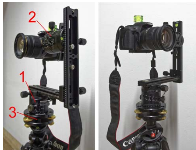
Fig. 1. View of the ILMD mounted on the panoramic head: 1 — rotator for rotation in the vertical axis; 2 — rotator for rotation in the horizontal axis; 3 — leveler allowing for the level setting by three independent screws.
