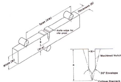
Fig. 4. Three-point bending CTOD test specimen.
