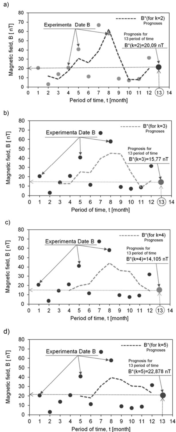
Fig.4 The results of measurements of the induction of magnetic field in the workplace of the operator (DMU 65 Mono Block): a) soothing constant  $k=2$ , b) soothing constant  $k=3$ , c) soothing constant  $k=4$ , d) soothing constant  $k=5$
