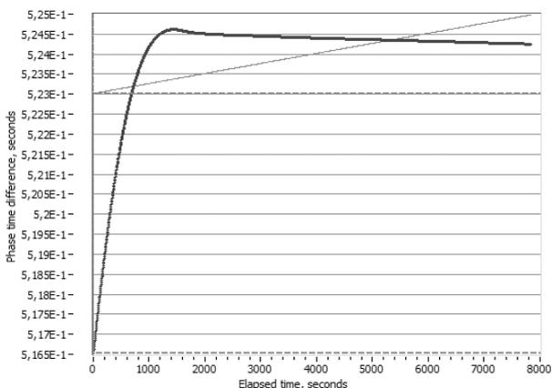
Fig.7. Phase time changes during the warm-up process of an OCXO thermostat after switching device on
