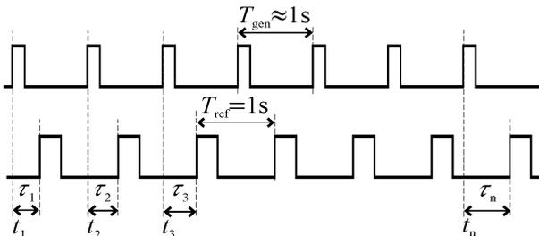
Fig.1. Basis for measuring the small frequency differences
