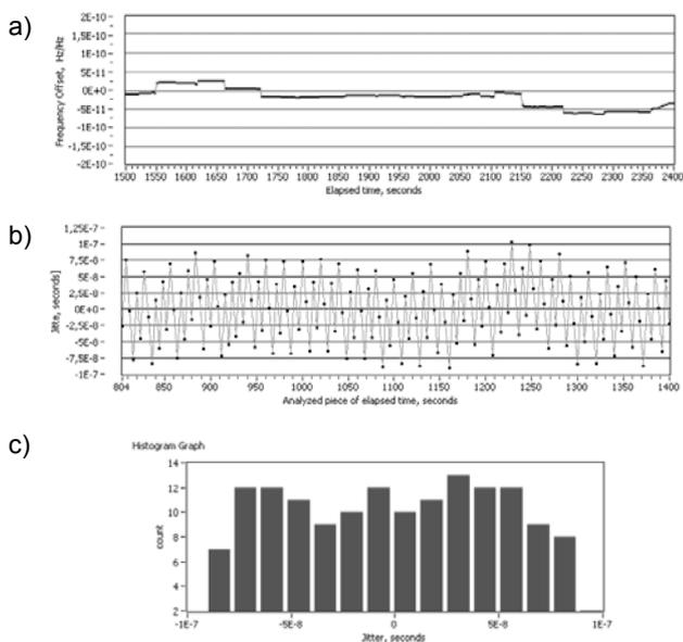
Fig.10. Measurement results obtained after the temperature stabilization and the generator is synchronized to the 1 PPS GPS signal with long averaging time equal to 5000 seconds: a) detuning measurement offset  $\delta f_{\text{gen}}$  in Hz/Hz, b) the sawtooth shape jitter in seconds, c) the uniform distribution shape histogram of the jitter
