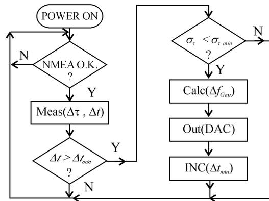
Fig.3. The synchronization algorithm for disciplining OCXO by the 1 PPS GPS signal
