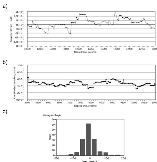
Fig.9. Measurement results obtained after the temperature stabilized and the generator is going to start synchronize to the 1 PPS GPS signal with short averaging time equal to 500 seconds: a) detuning measurement offset  $\delta f_{gen}$  in Hz/Hz, b) the jitter standard deviation  $\sigma_\tau$  in seconds, c) the symmetrical shape histogram of the jitter
