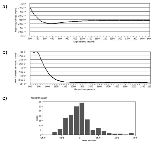
Fig.8. The warm-up process of an OCXO thermostat: a) detuning measurement offset  $\delta f_{gen}$  in Hz/Hz, b) the jitter standard deviation  $\sigma_\tau$  in seconds, c) the asymmetrical shape histogram of the jitter
