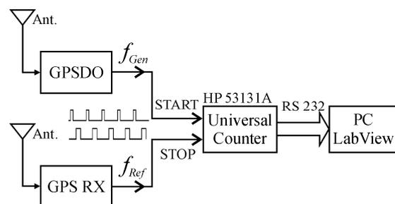
Fig.4. The flowchart of the measurement system for controlling the operation of the reference generator
