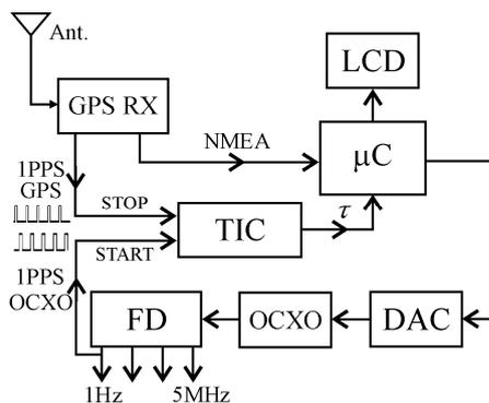
Fig.2. The flowchart of the OCXO generator synchronized to the 1 PPS GPS signal
