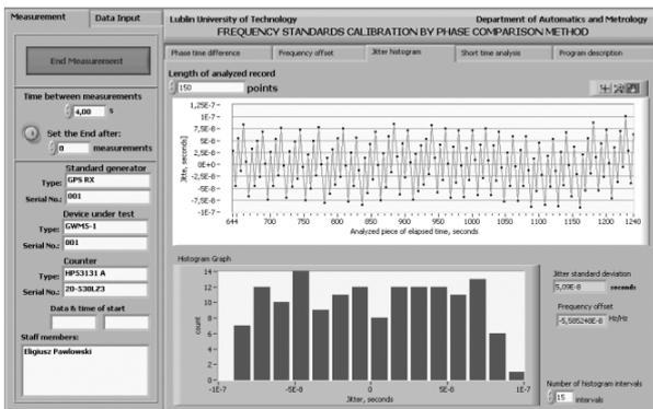
Fig.5. Front Panel of the LabVIEW measurement application for controlling the operation of the reference generator
